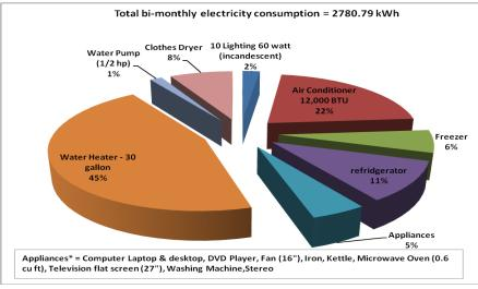
(a) Electricity Consumption With Air Condition
