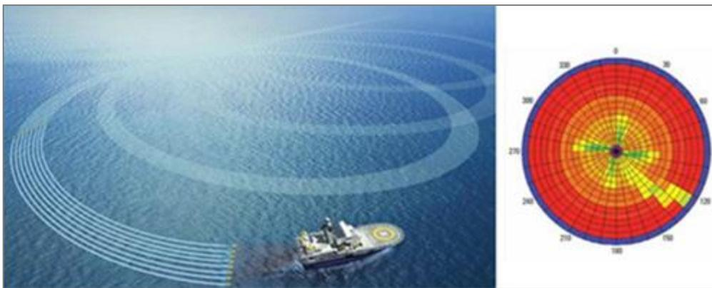
FAZ seismic data can be very expensive to acquire. In the marine environment, FAZ surveys using streamers must tow complicated paths, or use multiple vessels or shoot the survey multiple times. These techniques all imply additional cost, but the improved final image can justify the price tag by reducing drilling and development risk, especially in high-cost deepwater projects. FAZ data acquisition is about
