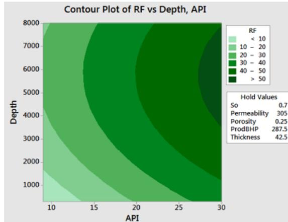
**Figure 3.4: Contour plot of RF for CO<sub>2</sub> injection**
