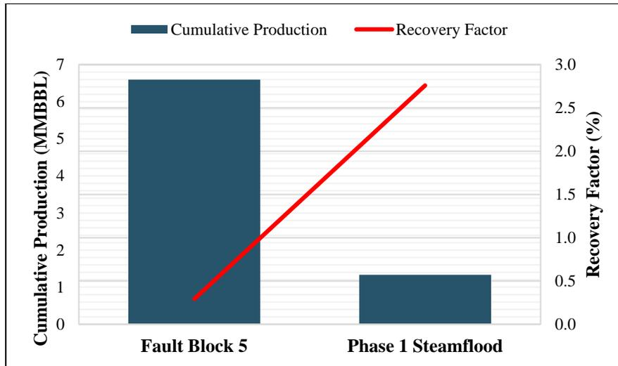
Figure 3.12: Primary Production for the Two Simulated Reservoirs
