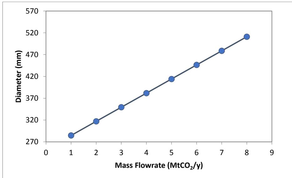
**Figure 3.2:** Estimation of pipeline diameter from mass flowrate.
