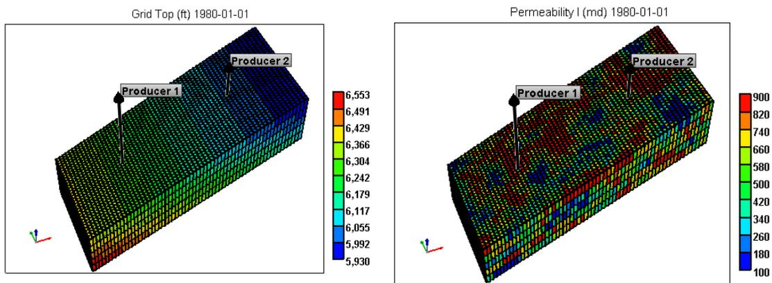
Figure 3.1: CMG 3D view of grid top (left) and permeability variation (right)
