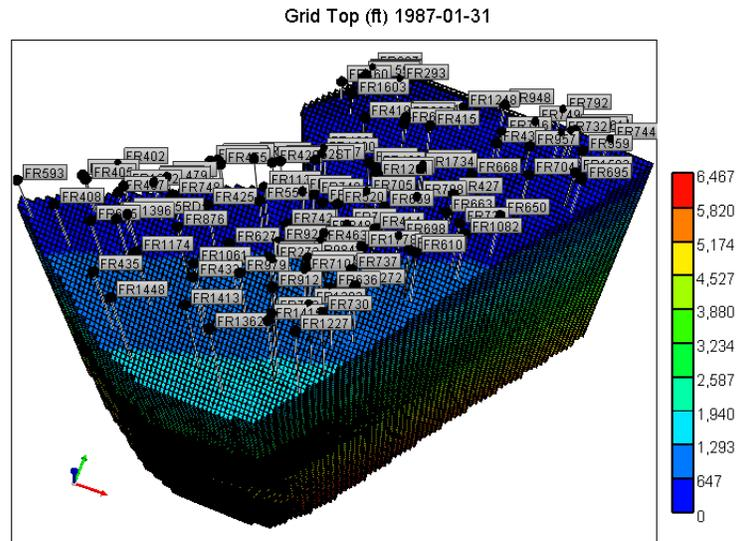
**Figure 3.10: Fault Block 5 CMG 3-D view of grid top**
