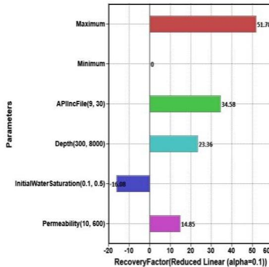
**Figure 3.3: Tornado plot of RF for CO<sub>2</sub> injection**
