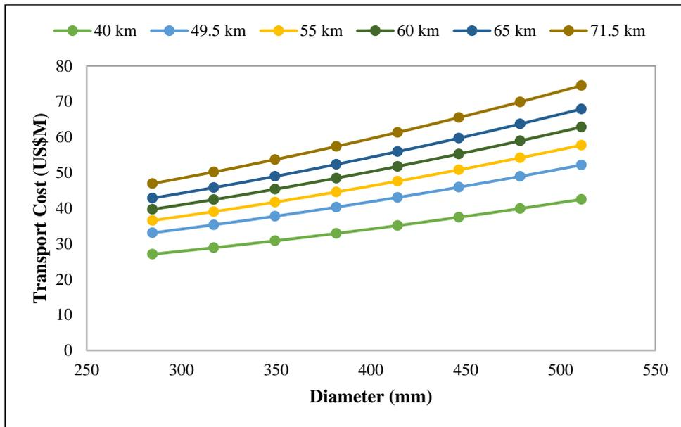
Figure 3.8: Sensitivity of transport costs to diameter and distance
