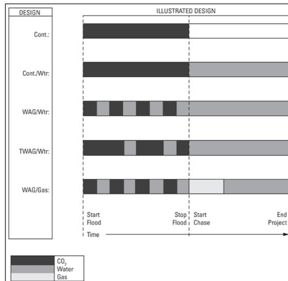
Figure 2.6: Schematic of various CO<sub>2</sub> flood-injectant designs in oil reservoirs. Retrieved from Jarrell *et al.*, (as cited in Verma, 2015)
