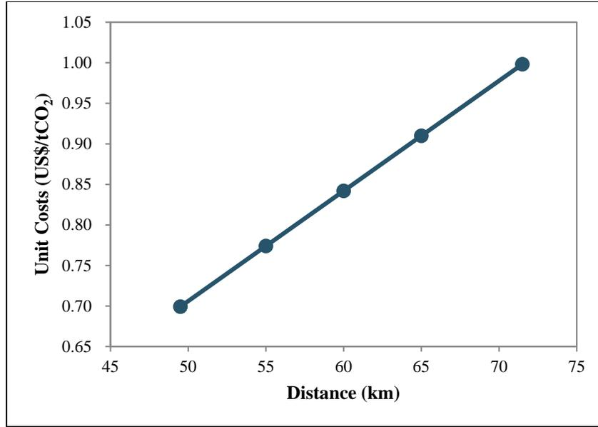
Figure 3.6: Total transport costs for T&T pipeline network with various distances
