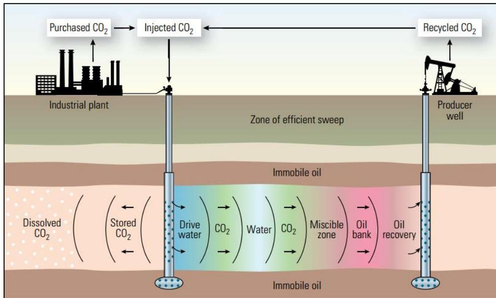
Figure 2.5: One-dimensional schematic showing the miscible CO<sub>2</sub>-EOR process. Retrieved from Ansarizadeh *et al.*, 2015
