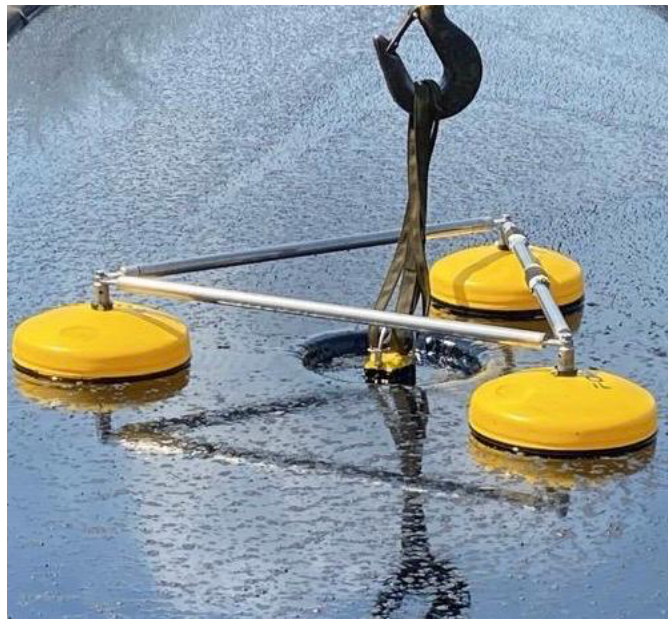
Skimmer component of the Rapid Deployment Skimming System (RDSS)
