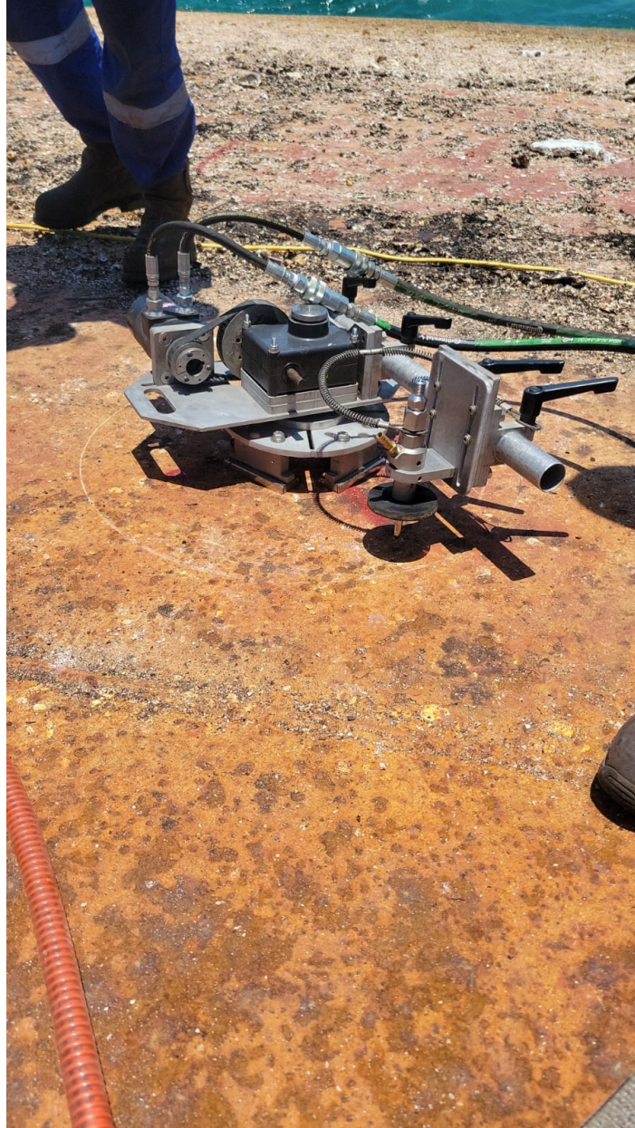
The locally acquired mobile water jet cutter used to penetrate the hull.
